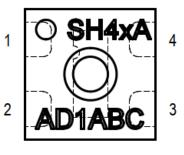
**Figure 12.** Pin assignment (transparent top view). Dashed lines are only visible if the sensor is viewed from below. The die pad is not directly connected to any pin.
